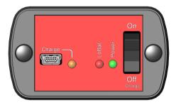
The green LED will now indicate that the RTI MAS-1 is powered ON. If the red "LoBat" LED lights up, it indicates that the battery voltage is low. Please recharge the RTI MAS-1 before measuring. See <u>Battery and charging</u> 6.
