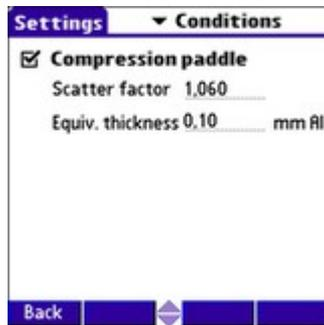
Figure 7. The scatter factor correction is added when you check the compression paddle box.
