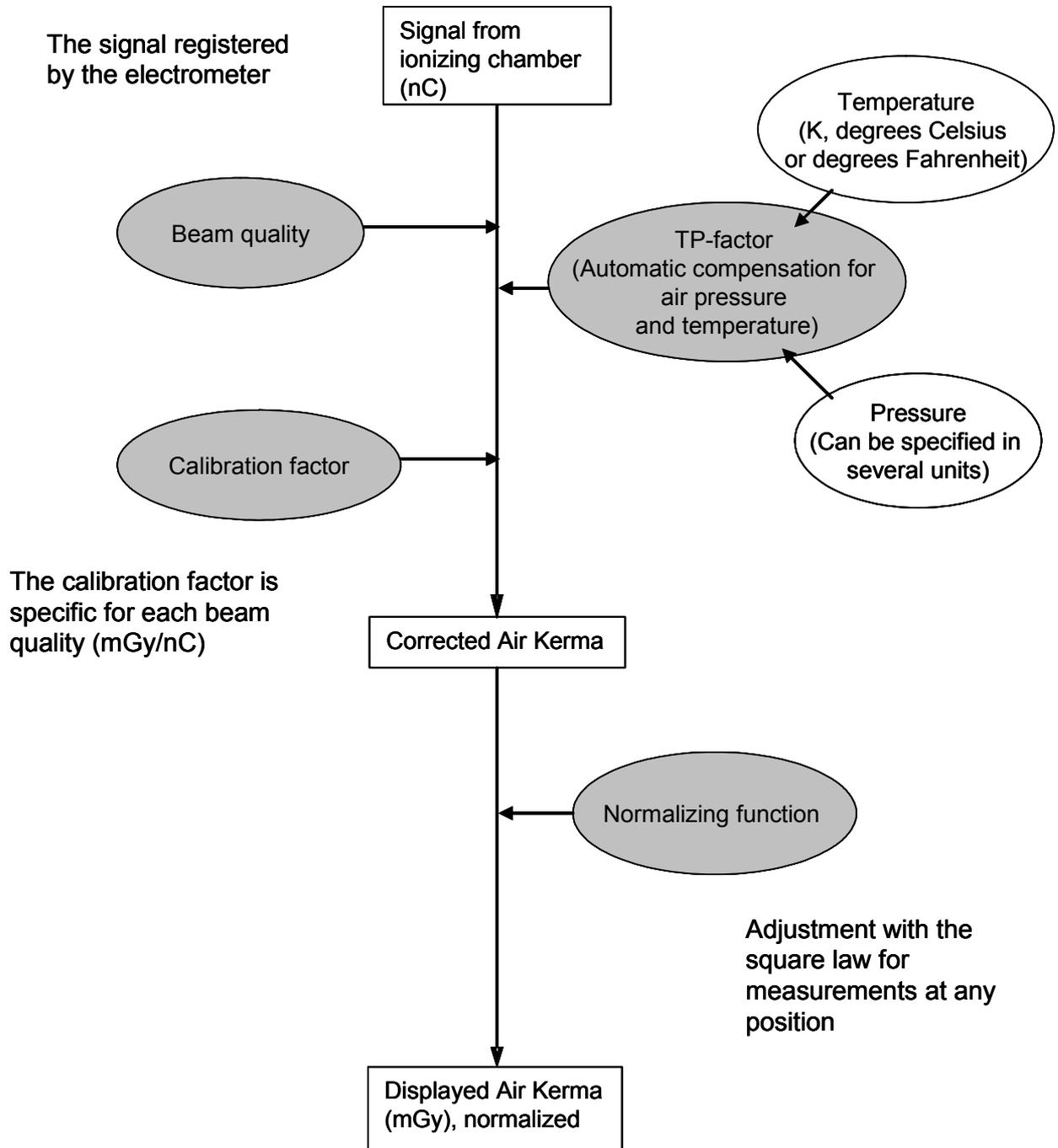
Figure 2. A flow chart of the handling of signal from the ionizing chamber to the Barracuda.
