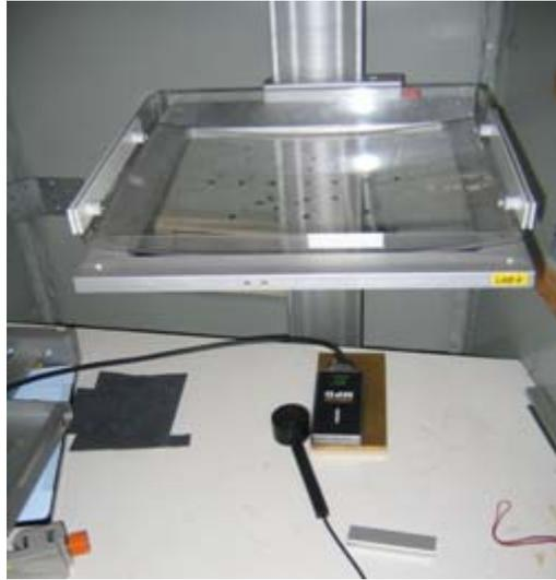
Figure 4. The Barracuda MPD and the Standard Imaging Magna 1cc positioned under the compression paddle (far from the detectors).
