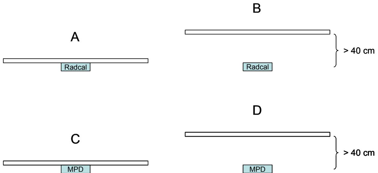
Figure 6. The thin white paddle is the compression paddle and the blue small rectangle symbolizes the detector. All measurements are made on a Sectra MDM.
