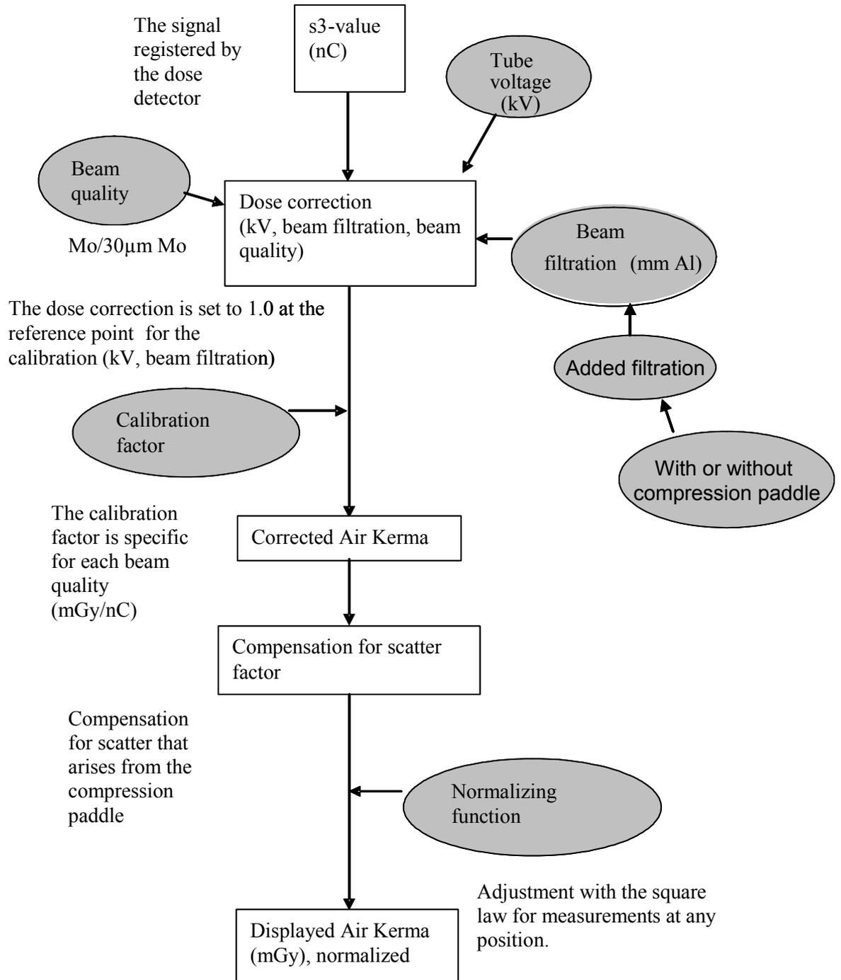
Figure 1. A flow chart of the handling of signal from the MPD to the Barracuda.
