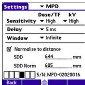
Figure 12. The setting of the normalizing function.
