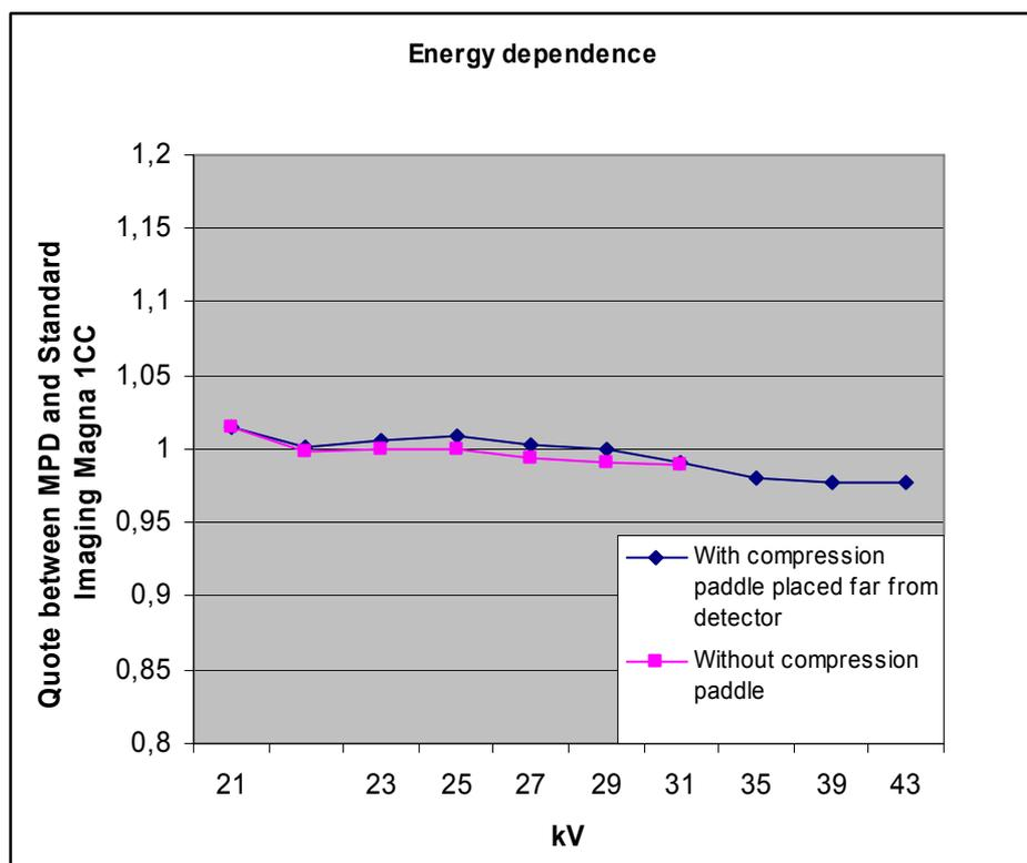
Figure 14. The energy dependence of the MPD compared to Standard Imaging Magna 1cc<sup>8</sup>.
