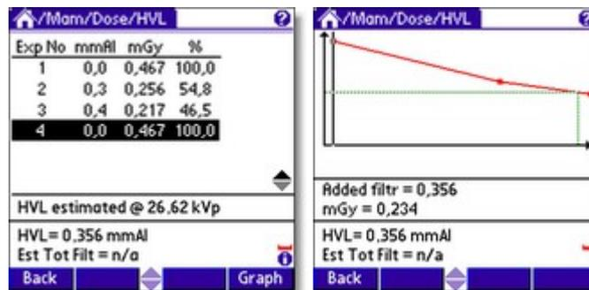
Figure 10a and b. The QABrowser display when performing a HVL measurement. By clicking on “waveform” the right figure appears.
