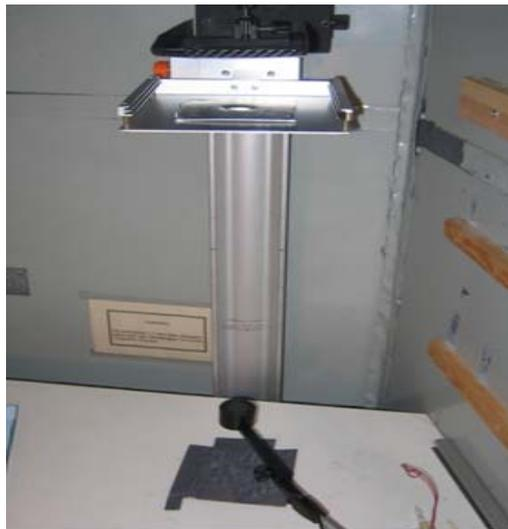
Figure 3. The Standard Imaging Magna 1cc without compression paddle. The Radcal 6M is used as the reference chamber.
