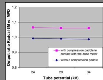
Figure 3. The energy dependence of the Radcal 6M compared to the MPD. When the ionising chamber is placed close to the compression paddle, a contribution of scattered radiation is added (with a magnitude of appr. 6 %).
