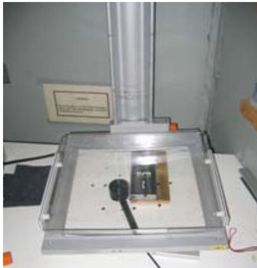
Figure 5. The Barracuda MPD and the Standard Imaging Magna 1cc positioned under the compression paddle (close to the detectors).
