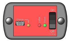
The green LED will now indicate that the MAS-1B is powered ON. If the red "LoBat" LED lights up, it indicates that the battery voltage is low. Please recharge the MAS-1B before measuring. See <u>Battery and charging</u> 6.
