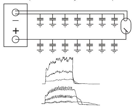
Selected values: 100 kV, 80 ms and 10, 25, and 50 mA. The upper part of the right picture shows the radiation intensity response from the detector. The lower part of the figure shows the tube current measured with MAS-1B. Note especially the last part of the exposure. Large mAs errors can be made if this part cannot be avoided. The left picture shows that the high voltage cables act as capacitors and can influence the mAs measuring result.
