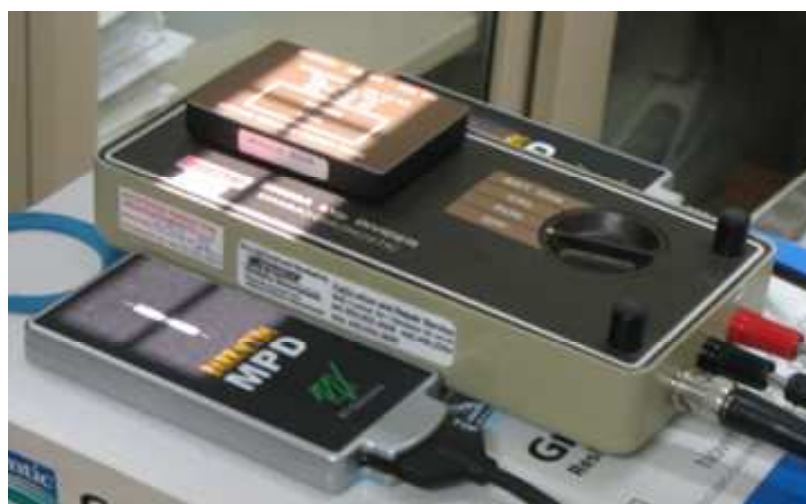
Figure 1b. The Barracuda MPD and the Triad System model 10500AT consisting of the 35080B non-invasive divider using the 37946C mobile filter pack. The 35080B sensor area was placed in the center of the field and 90° to the anode cathode in order to measure and display accurate results. The check filter of the MPD was used to correct any field symmetry problems in the ratio allowing the Barracuda to measure and display accurate results. This is a unique feature and advantage of the MPD.
