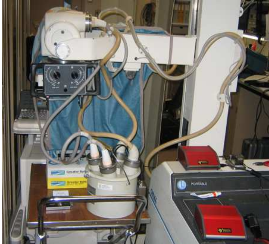
Figure 1a. The RadCal HV-1 invasive voltage divider connected to the Barracuda SEM module.
