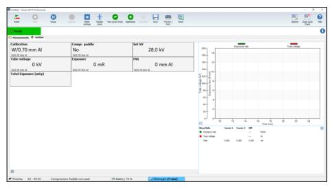
A **Position Check** in the W/0.7 mm Al beam quality should be performed before the Combo mode is run.
