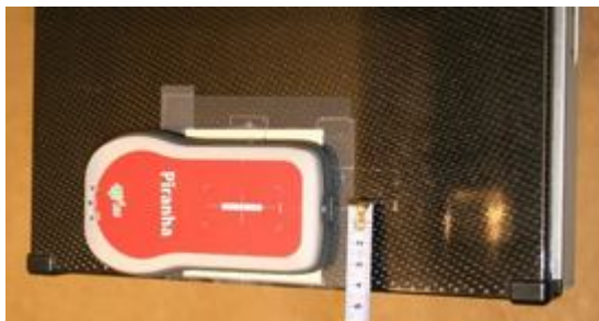
Figure 1. Detector positioning for Quick HVL measurement
