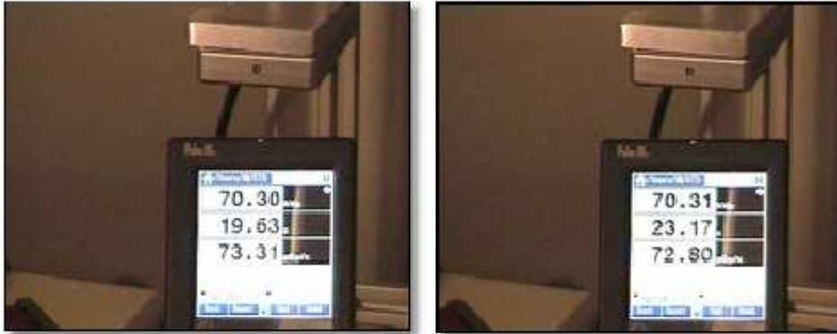
The dose rate is now much lower. The added filtration does not affect measured kVp at all.
