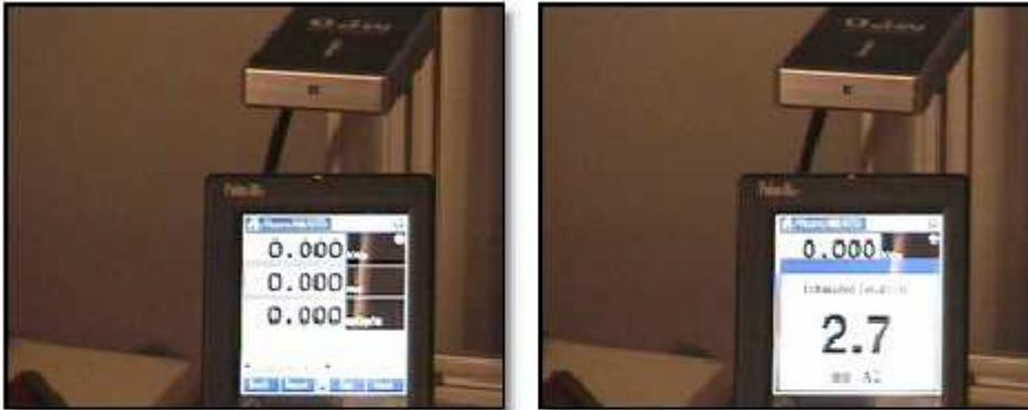
The fluoro is started and the total filtration is estimated and automatically displayed during two seconds.
