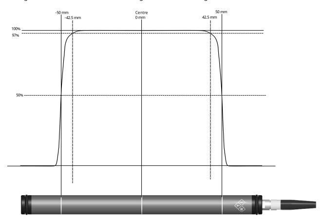
The effective length and the rated length are given as defined by IEC 61674 (Ed.2, 2012). Within the rated length (85 mm) the sensitivity is within  $\pm 3\%$  of the sensitivity at the center of the chamber. The effective length is given at the position where the sensitivity is 50% of the sensitivity at the center of the chamber.
