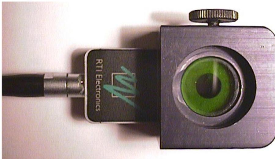
**Figure 3** The basic light detector which includes the CIE filter house.
