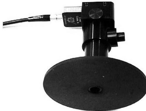
*Figure 4* The monitor adapter with light shutter and ambient light shield.
