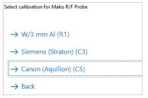
When using the Mako R/F Probe in CT applications, there are only 3 options, a universal beam quality (W/3 mm Al, which can be used for all CT manufacturers/
