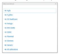
When using the Mako Mammo Probe, calibrations are grouped according to X-ray manufacturer and model, with an additional 'generic' list if required. Quick Check adapts automatically to your selection.
