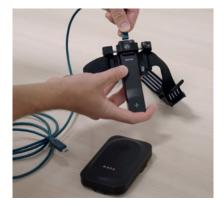
2) Connect the Mako Probe to the Mako Base Unit via USB cable.
