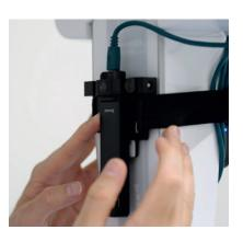
5) Loosen the locking mechanism to make fine adjustments to the Probe position, then tighten to fix.
