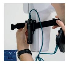
3) Use the strap and clip to place the Mako Probe into the correct position for X-ray exposure.
